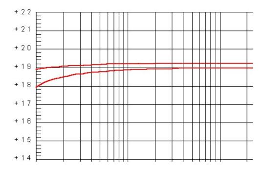
Distortion vs output watts into 8 ohms at 1 Khz:
