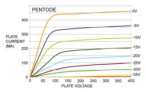
The behavior of an ordinary Jfet or Mosfet is very similar. As with the Pentode, the current flowing from Drain to Source in a Fet will flatten out as the voltage between those pins increases. In this regard Mosfets have a similar shape to the curves of Bipolar transistors, except that Bipolars use input current for control instead of voltage.
