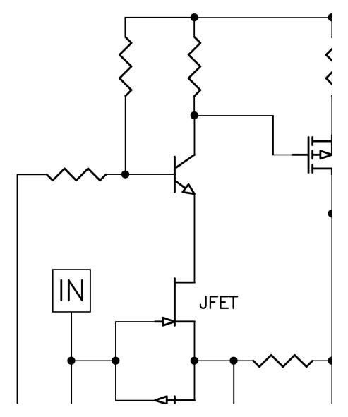
It is current biased by a negative 60 volt supply rail through a P channel Mosfet rated at 500 volts, 40 amps and 890 watts. This arrangement is unique in that the SIT is given a single-ended Class A bias current by the P channel Mosfet which is allowed to make a smaller contribution to the output, typically about 20%. This is seen on the right hand side of the schematic where the output goes through two sets of power resistors and capacitors.
