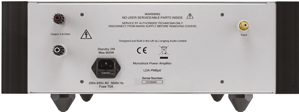
Loudspeaker binding posts, a single RCA input plus an IEC mains input take up the back of the LDA P6. Simple - but effective. There is no balanced XLR input.
