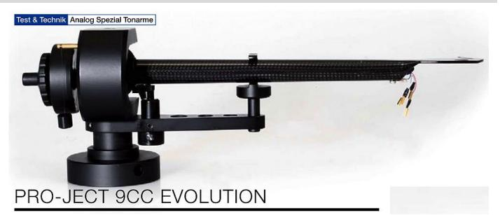
Arm tube and headshell are made of a single piece of carbon, while the arm tube itself is conically shaped. 9cc Evolution utilises inverted ball bearings made from high-grade stainless steel. Azimut can be adjusted through rotation of the arm tube.
