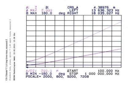
In the photo/plot is shown the comparison of a HiFi-Tuning Ultimate<sup>3</sup> 6,3 x 32 mm ; T 1,6Amp. fuse with a standard fuse glas/spiral T 1,6Amp.
